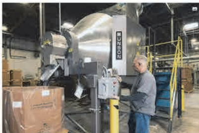
An operator programs mixing cycles at a frame-mounted control panel.
